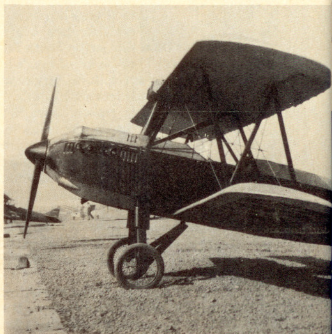
Early International F-17 with Curtiss OX-5 engine. The pilot's small cockpit is invisible in this view because of the flat top of the octagonal fuselage. Note the no-brakes wire wheels and the radiator built into the upper wing.
